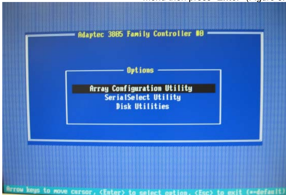
Figure 6-3 Array Configuration Utility
